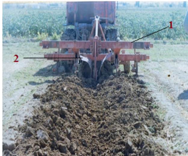
Fig. 2. Operation of the ploughing unit with front housings arranged in a sheet pattern without plungers: 1 – frame; 2 – front plough bodies
