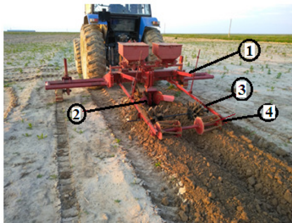
Fig. 6. Test sample of a combined tillage unit for melon crops in operation: 1 – frame; 2 – front plough bodies; 3 – rotary tillage implement with spherical knife elements; 4 – plank rink
